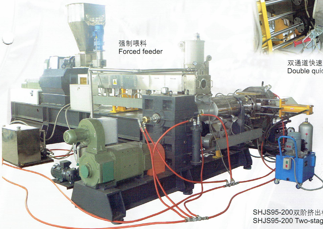
风冷模面热切粒机组 Air-cooling hot face pelletizing line
